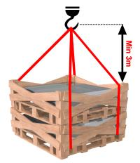
THE LIFTING HOOK SHOULD BE NO LESS THAN 3M ABOVE THE LID
